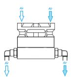
Smartshift Manifold is to be used if the air is to be directed out on the sides and not directly in to the tool, mounted on the Tool Holder (TH).
