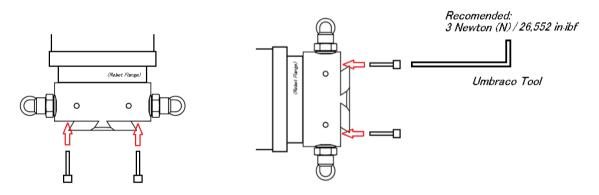
If there is no accurate fit to the Robot flange, contact Smartshift Robotics AS for adaptor to fit the connection.
